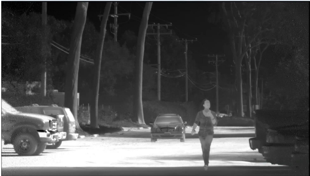
Figure 2. MWIR image of CS-3 ROIC hybridized to nBn detector material operating at 150 K
