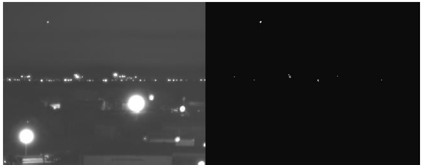
Figure 2. SWIR night image of distant highway and airplane (left) and motion computation binary image (right) showing auto-detection of vehicles and airplane
